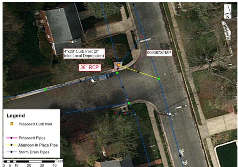
Figure 10: Dogwood Drive Storm Drain Pipe Realignment
