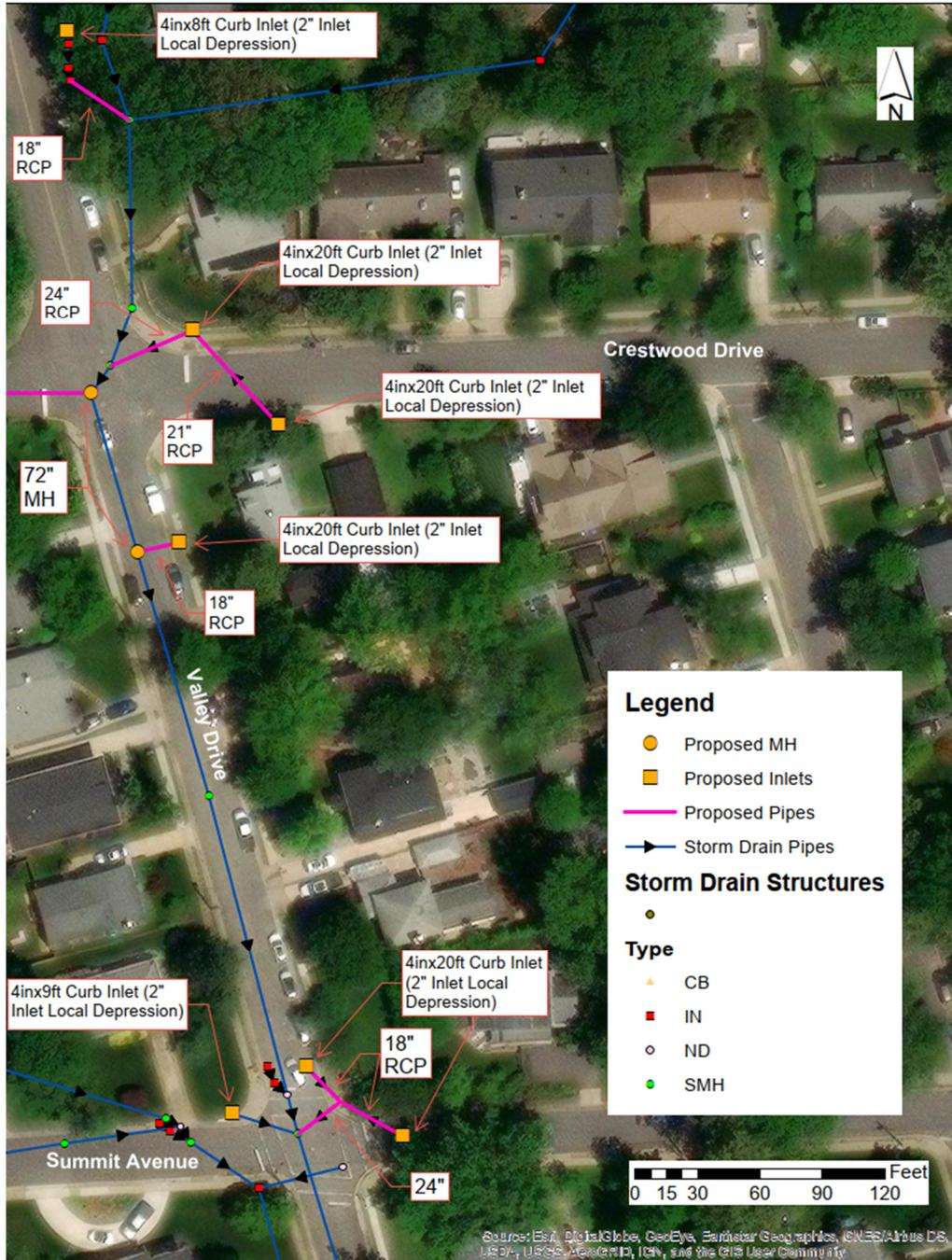
Figure 12: Valley Drive Inlet Upsizing and Storm Drain Pipe Locations
