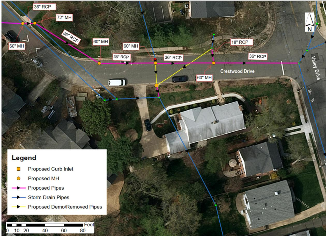
**Figure 7: Proposed Storm Drain System along Crestwood Drive**
